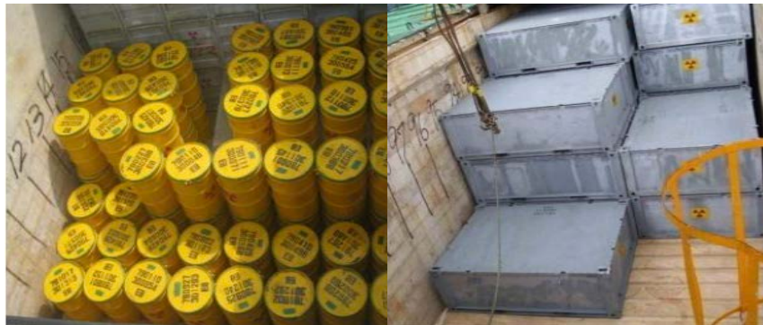
Fig. 6: Left, 55-gallon drums In a Storage Trench; Right, 0.914 m by 1.219 m (3 feet by 4 feet) Galvanized Steel Containers in a Storage Trench, as of November 2011
